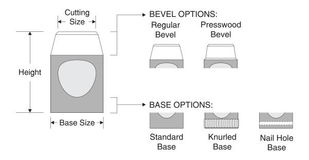
Bevel and base options may be combined. Extra charges apply for bevel and base options. All Self Cleaning Punches are available in Heavy Duty, Through Hardened Tool Steel.
