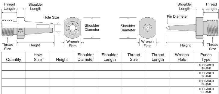
\* Note: For threaded shank pin point punches enter pin diameter in this column.
